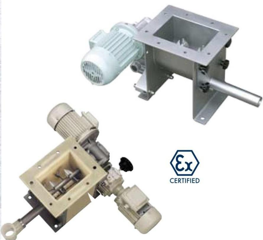
**MBF Micro-Batch Feeder** for continuous volumetric feeding of powdery or granular materials consist of a body entirely manufactured from stainless steel (optionally steel-reinforced SINT® engineering polymer), a horizontally mounted rotating agitator tool, a feeder screw beneath the agitator tool, a feeder pipe enclosing the protruding feeder screw, one drive unit each for agitator and feeder screw.
